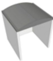
Soffitto a botte Barrel vault ceiling
